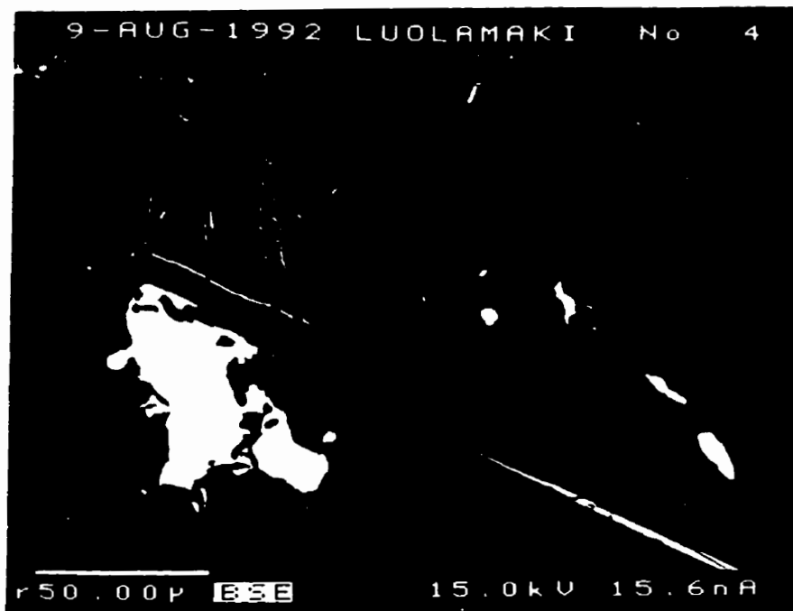
Fig. 4.16. BSE images of feldspar from Luolamäki: (A) (Rb,K)-feldspar (white) between grains of lepidolite (black), showing a compositional gradient from microcline (grey) ; (B) laths of lepidolite (interlayer apatite - white) in microcline (grey) associated with Rb-rich feldspar (white) and surrounded by Rb-poor K-feldspar (dark grey).
