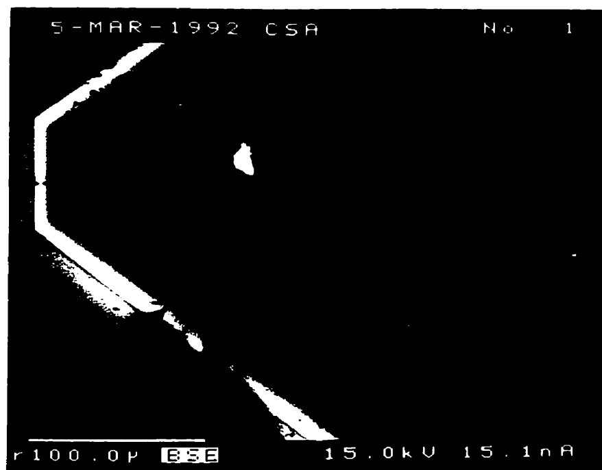
Fig. 4.35. BSE images of cesian analcime from Tanco, Manitoba: (E) Cesium-exchange along a fracture in cesian analcime, generating pollucite-like compositions; (F) The Cs-rich core of sample CsA, with minor analcimization along fractures.
